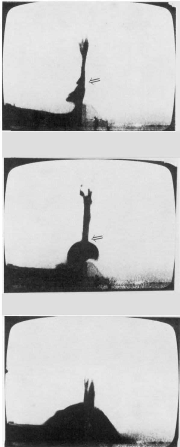
FIGURE 13. Impact sequence showing the overflow and formation of a shock. Theory accounts well for fluid motion below the height indicated by the arrows. Particles in the liquid jet above this are essentially in free flight and reach a height about three times that of the tank.
